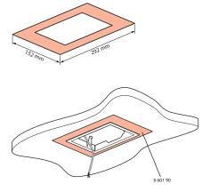
This accessory is only installed with flush-mounting frame 6 601 90 and URA NEXT self-contained emergency lighting units.
