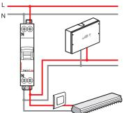
The branch can be joined in the electric cabinet, on the switch or in a junction box.
