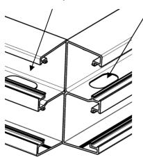
Funds of the bodies provided with holes for fixing, facilitating the upgrade of the trunking (balance/slope)
