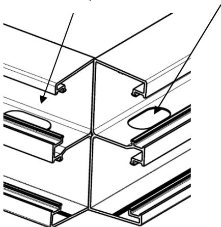
Funds of the bodies provided with holes for fixing, facilitating the upgrade of the trunking (balance/slope)
