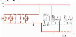
For a 1 "NO" single pole or a 2 "NO" 2-poles latching relay
