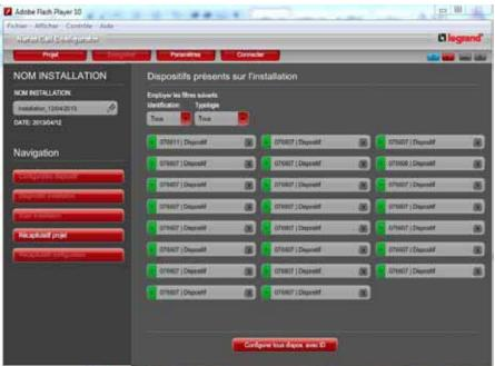
(7) Enter the IP address of the configuration kit (default address: 192.168.1.35 and default password: 12345) to connect the software to the system. Click on "Save data" to save the modifications then click on "Project summary".
