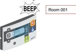
The door unit signals the call from the room (indicating the room number on the display unit) and emits an audible alarm.
