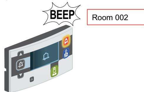
The door unit signals the call and emits an audible alarm.
