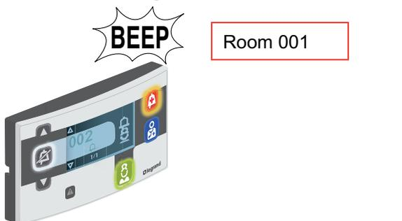
The door unit signals the call from the room (indicating the room number on the display unit) and emits an audible alarm.
