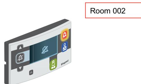
The door unit signals the call. The audible alarm is cut off.
