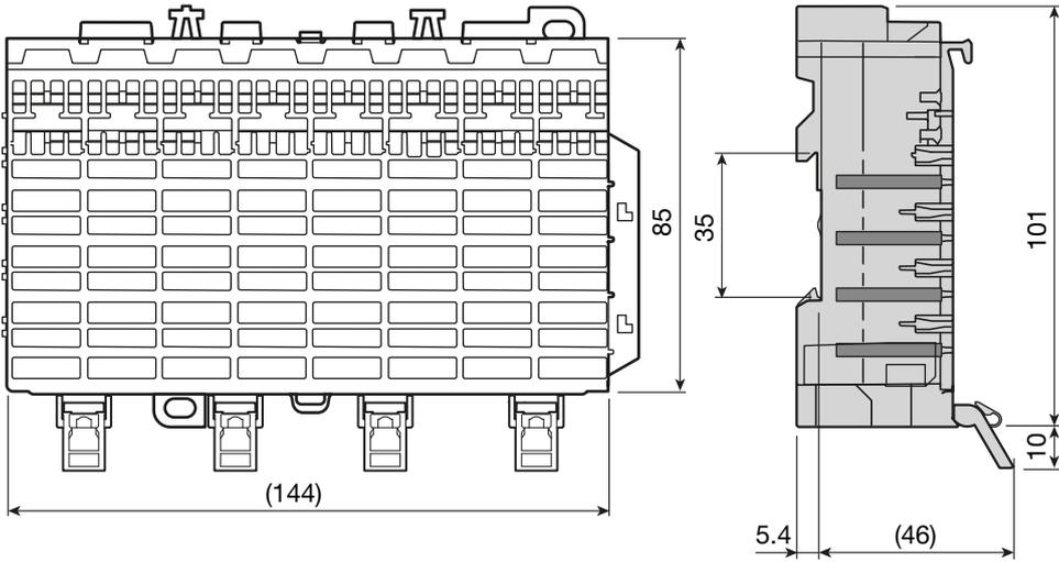
**6-module socket ZLSP906 and additional socket ZLSP926 including end piece**
