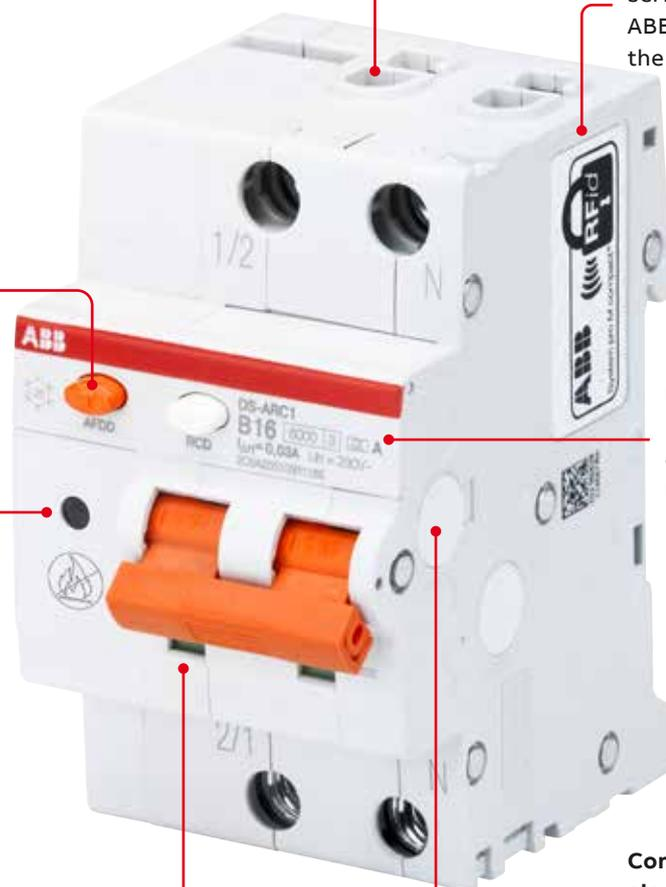
The DS-ARC1 is the new 1P+N Arc Fault Detection Device (AFDD) with an integrated residual current circuit breaker with overcurrent protection (RCBO) in only three module width. The series offers a complete protection against arc faults and overvoltage, reducing the risk of fire. The integrated RCBO is adding protection against overcurrent and earth fault currents: compact solution for a complete protection of people and valuable assets.
